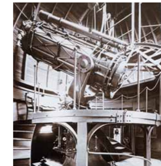
Reflecting telescope at University of Heidelberg (1906) The world’s first large reflecting telescope SCHOTT provided the reflector base of 720 mm.
